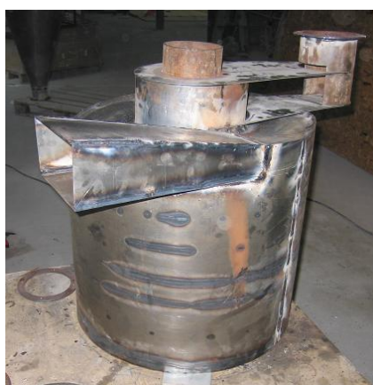
Figura 1.2.4 a, b - Model experimental simplificat de sistem modular de depoluare a gazelor industriale - Exhaustor
