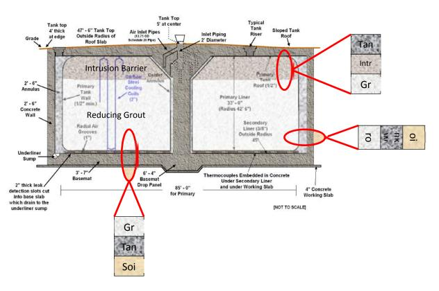
FIG 16. One dimensional conceptual model constructed to evaluate cementitious barrier performance associated with a waste tank.
