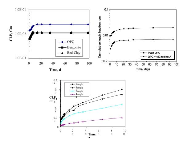
FIG. 4. Cumulative leached fraction from modified cement matrices.
