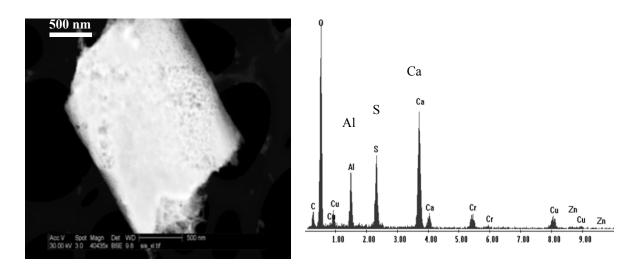
FIG. 12. STEM-in-SEM/EDX microanalysis of ettringite (carbon comes from the sample holder, Cu from the copper grid, and Cr from the detector).
