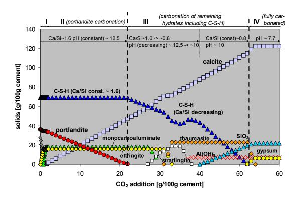
FIG. 17. Effect of carbonation on the mineralogy of hydrated ordinary Portland cement.
