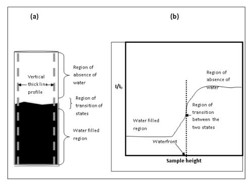
FIG. 8. (a) Schematic diagram of a radiograph showing a water front within a cylindrical mortar sample and (b) Determination of the water front height from the resulting curve of intensity as a function of sample height.
