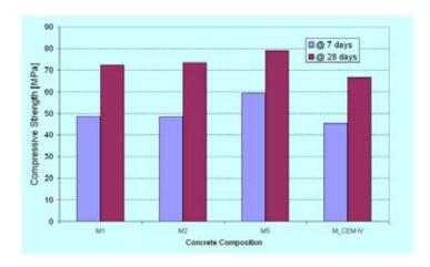
FIG. 6. Results of compressive strength measurements for 4 compositions for 2 time periods.
