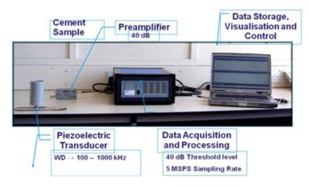
FIG. 10. Acoustic emission technique used in current CRP.
