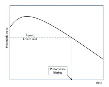
FIG. 18. Representation of durability and the relationship between parameters, time in service and performance lifetime.
