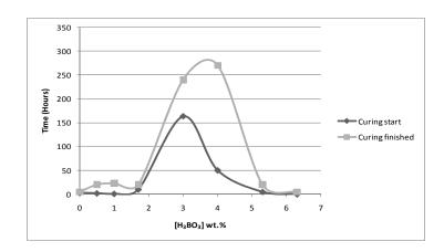
FIG. 2. Impact of borate waste content on time to initial and final set.
