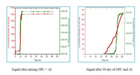
FIG. 11. Cumulative number of AE hits and associated ABS energy detected during the AE monitoring of the BFS/OPC samples with encapsulated Al.
