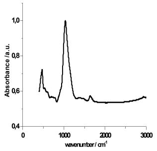
FIG. 13. Infrared spectra of SIAL® matrix sample.
