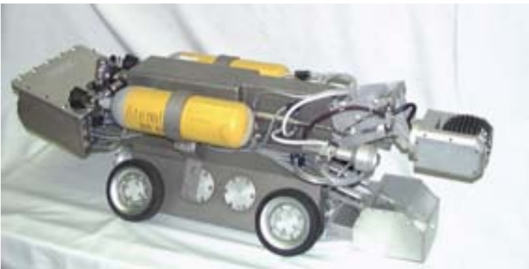
FIG. 7. A pipe inspection and removal trolley of type PCK-60, used in the Czech Republic.
