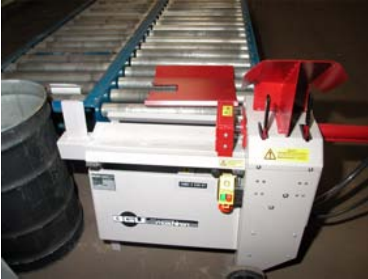
FIG. I-7. Underground pipeline decommissioning in Belgium: size reduction of the pipe ducts. Courtesy: Belgoprocess.
