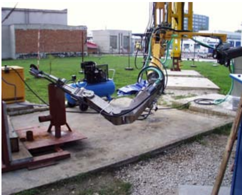
FIG. 19. The DENAR-41 manipulator during mock-up testing, Slovakia.
