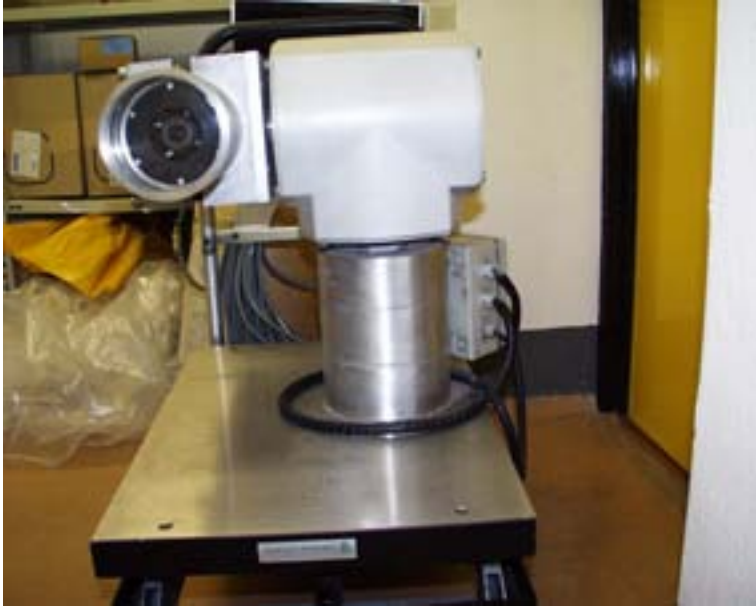
FIG. 18. The ALADIN camera in use at the A-1 nuclear power plant decommissioning project, Slovakia.
