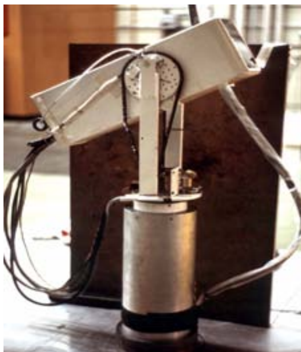
FIG. IV-2. The TV camera with custom made swivel and tilt joints used at Lucens.
