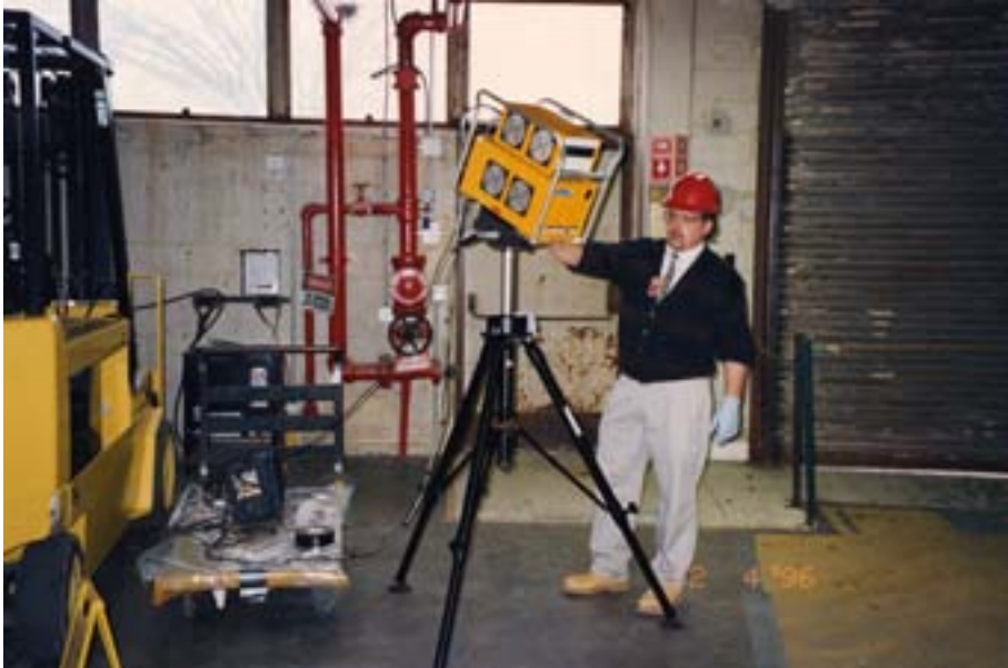
FIG. 17. A GammaCam as used for the gamma radiation field at the CP-5 reactor facility, Argonne, Illinois. Courtesy: Argonne National Laboratory, managed and operated by the University of Chicago for the USDOE under Contract No. W-31-109-ENG-38.
