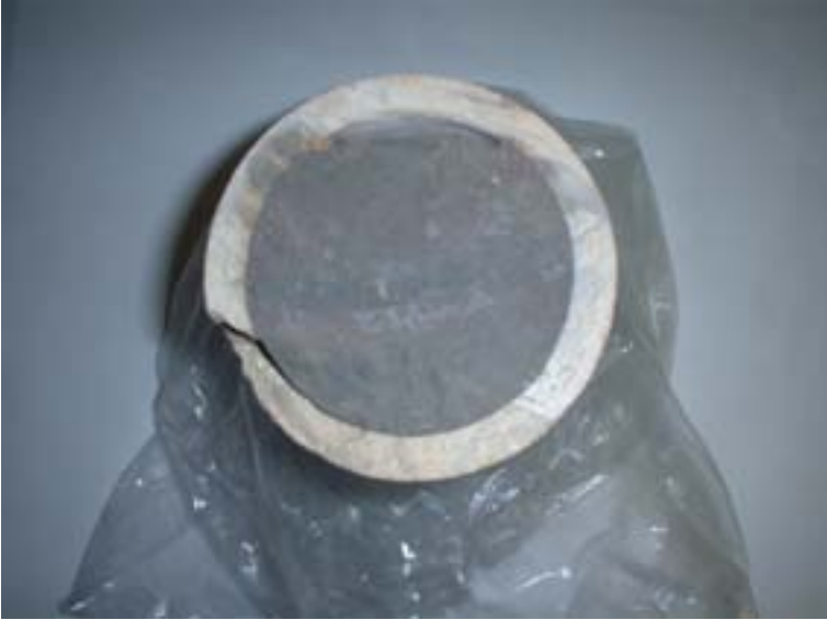
FIG. V-3. Grouted drain section at Harwell, UK.
