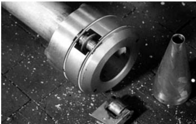
FIG. IV-5. The in-pipe cutter used at Lucens for CO 2 pressure tubes.
