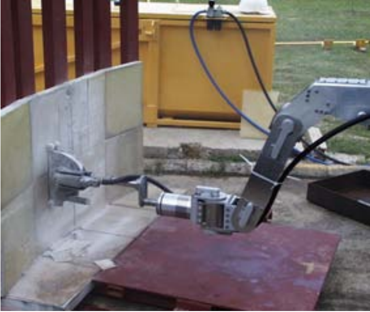
FIG. VII-5. Mock-up testing of the cutting of underground tanks at the A-1 nuclear power plant at Jaslovské Bohunice.
