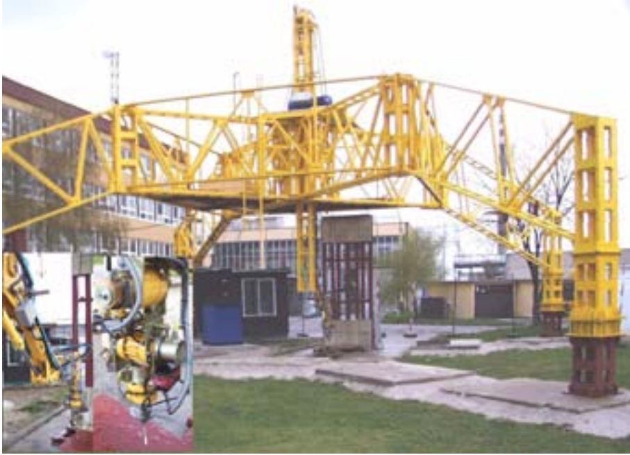
FIG. 20. Full assembly of the DENAR manipulator during mock-up testing, Slovakia.
