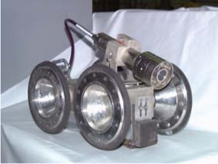
FIG. 6. A pipe characterization trolley of type PVK-3, used in the Czech Republic.
