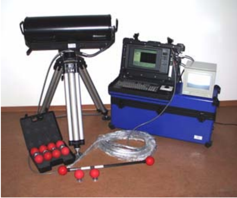
FIG. 16. A 3-D laser scanner in use at the A-1 nuclear power plant decommissioning project, Slovakia.
