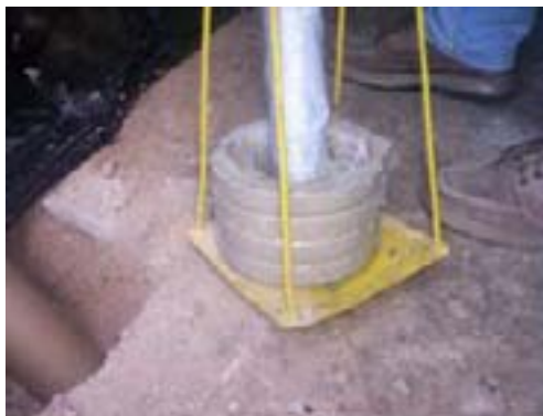
FIG. IX-2. Dose rate monitoring on a floor surface at INOR, Havana.
