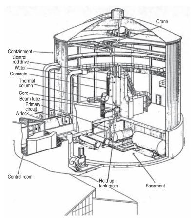
FIG. I.C-3. Cutaway drawing of DR-2.
