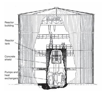
FIG. I.C-4. Cutaway drawing of DR-3.
