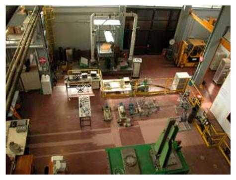
FIG. 16. Former hall of the RB-2 reactor, now converted to an experimental test laboratory for structures and components at ambient and high temperature.
