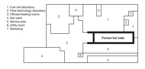
FIG. I.C–5. Schematic of the partly decommissioned hot cell facility.
