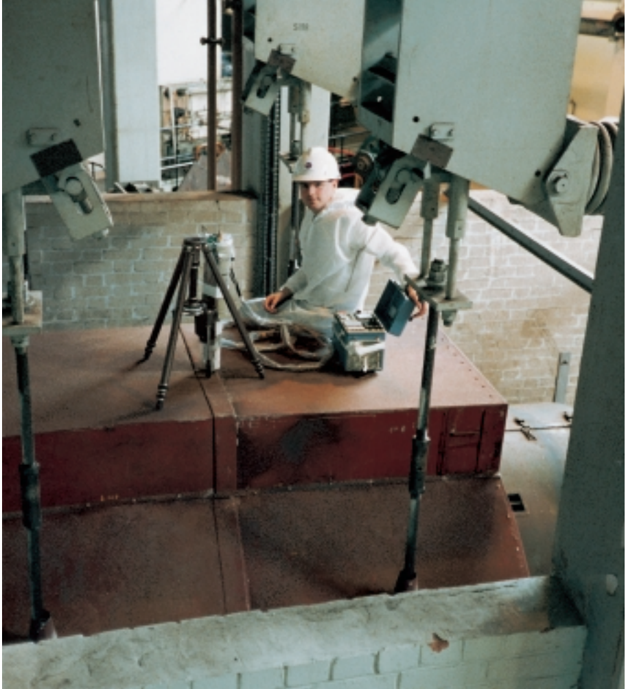
FIG. 8. In situ \gamma spectrometry in decommissioning (Magnox Electric, UK).
