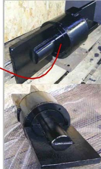
nonlinear elastic telescopic device with radial friction
