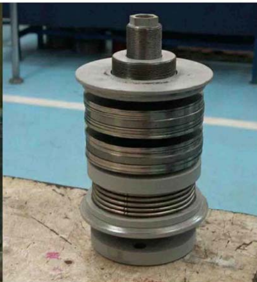
SERB-HP-160 Damper for Hydraulic shocks elastic room of SERB device
